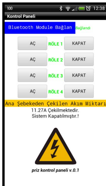
Figure 5. System is terminated after the current value is more then the limit value
