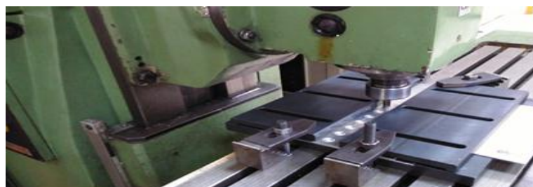
Figure 3. The milling machine used for friction stir spot welding process
