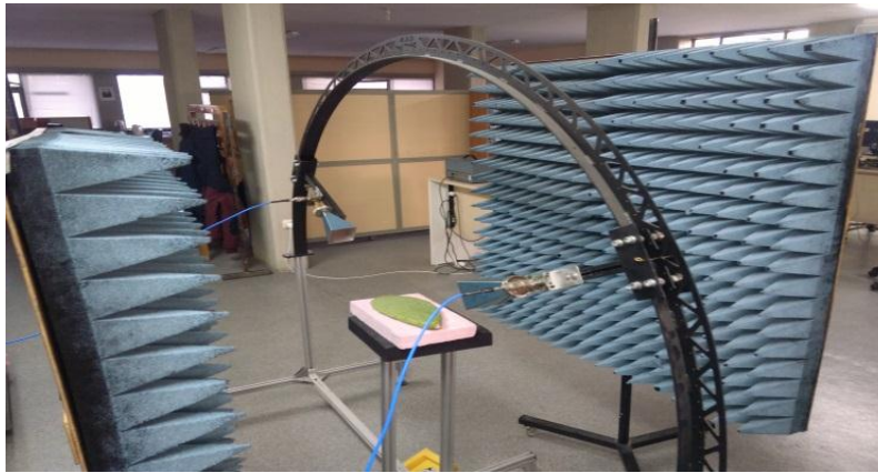
Figure 9. Arch free space measurement set up
